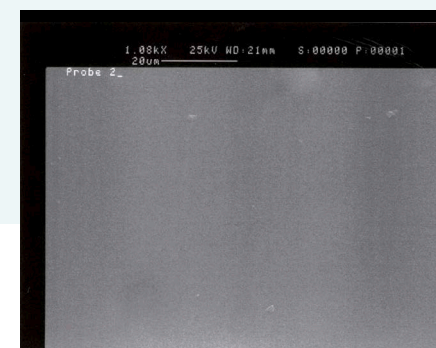
SEM* image of the RAUMEDIC PU ventricular catheters**:
